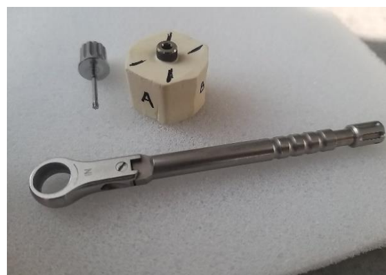
Figure 8. The Bredent Blue Sky implant fixed in a plaster hexagon.
