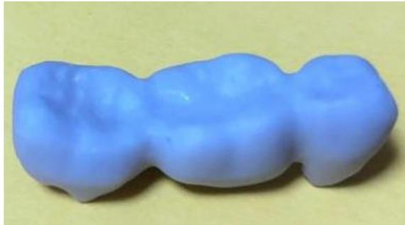
Fig.4 Ceramic bridge after removal from the milling chamber
