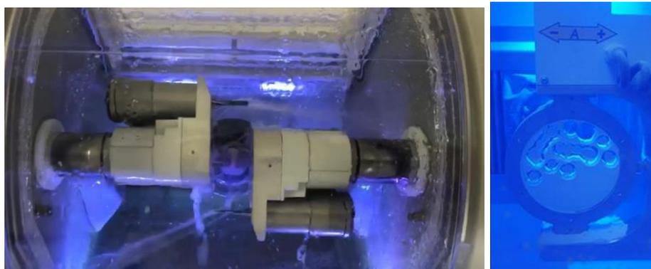
Fig.3 Milling the ceramic block
