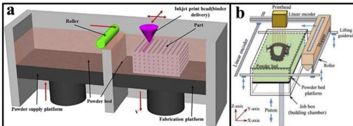
Figure 6. Powder binder printer principles (Mostafaei A-2017)
