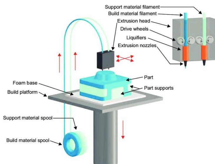
Figure 4. Fused deposition modelling (Heras ES – 2017)
