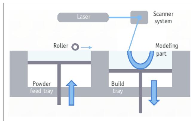
Figure 5. Selective laser sintering principles
