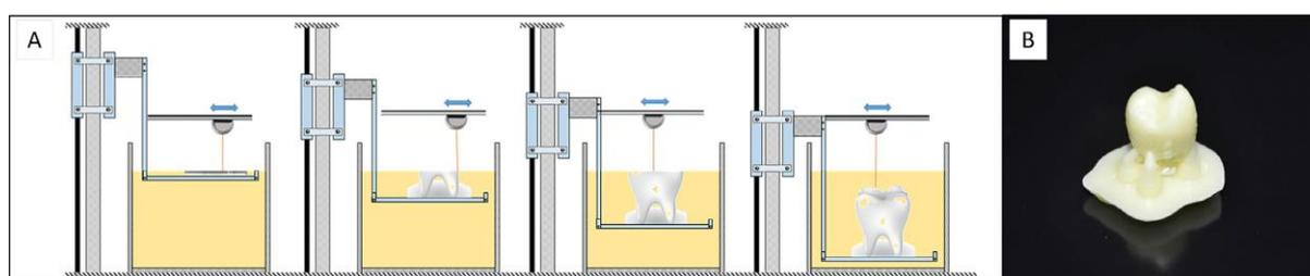
Figure 1. Stereolithography printing. (A) Layer by layer printing process. (B) An example of a crown printed with stereolithography prior to removal of supports and polishing [Sakly A, et al-2014].
