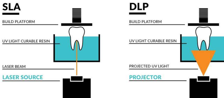
Figure 3. Differences between SLA and DLP
