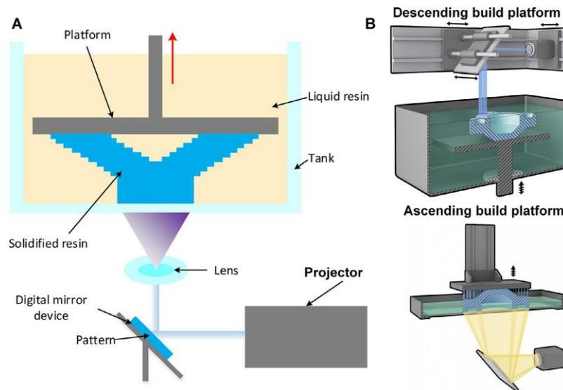
Figure 2. Digital light projection (DLP). (A) Schematic of the printer components and printing procedure. (B) Demonstration of two kinds of platform movements in DLP method [Pan Y-2012] .
