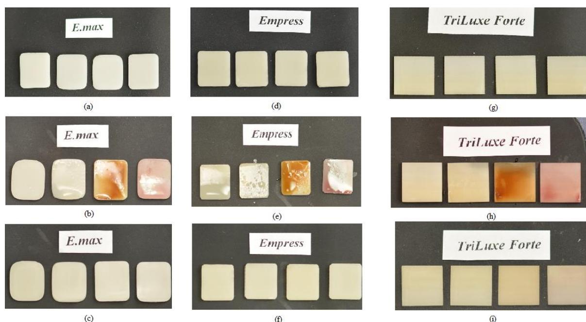
Figure 3. (a,d,g) Ceramic discs at the beginning of the experiment before immersion; (b,e,h) ceramic discs after storage in solution before washing; (c,f,i) ceramic discs after 4 weeks of storage in different storage liquids.
