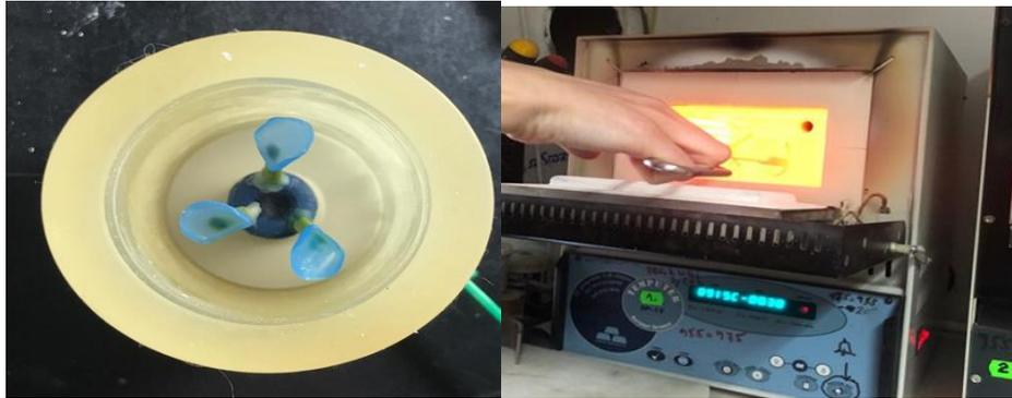
Fig.2 Investing and mold realization
