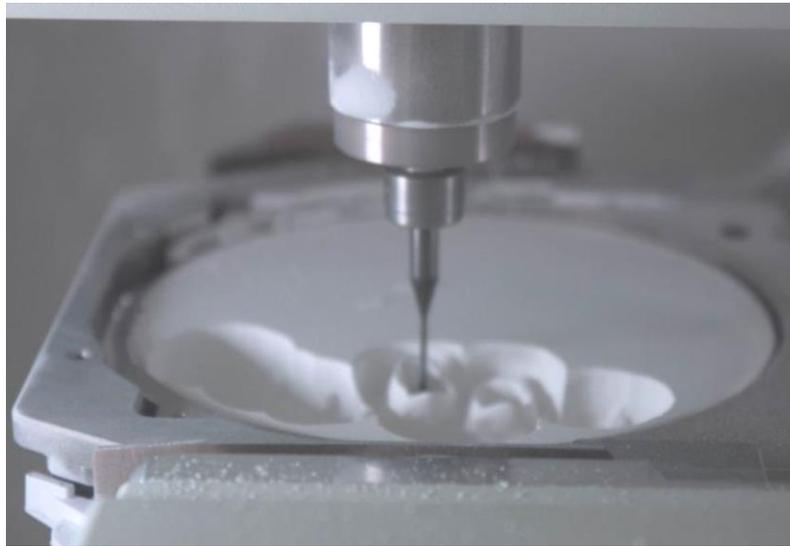
**Fig.8 Milling of ceramic framework**
