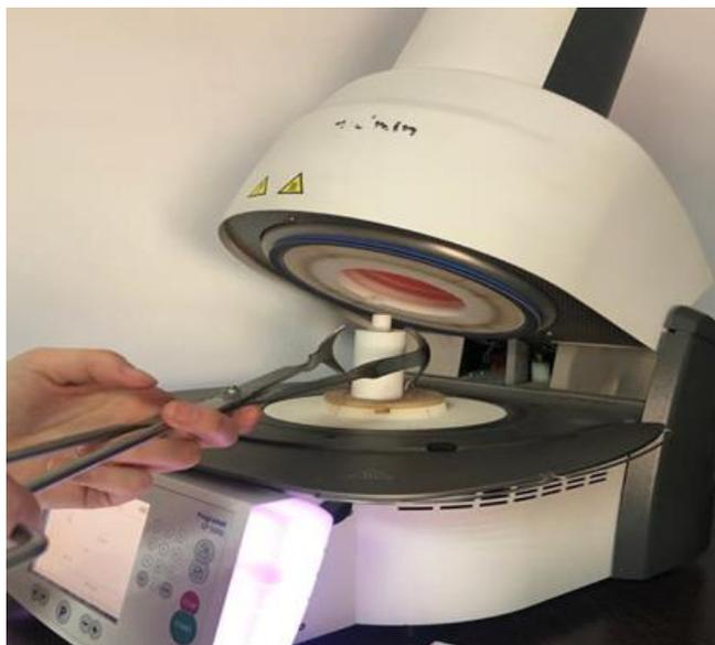
Fig.3 Pressing the ceramic in the mold
