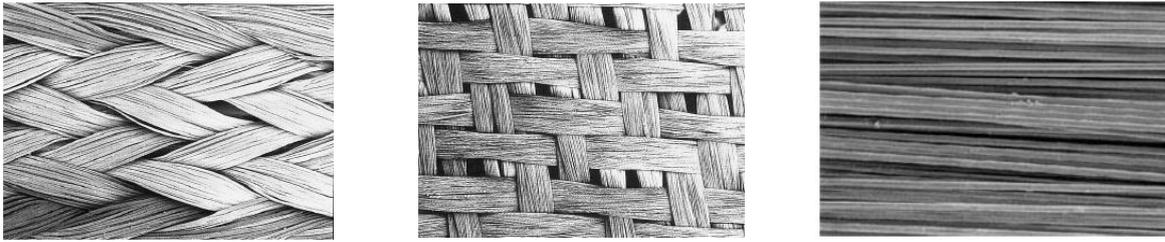
**Fig. 1. Types of reinforcing fiber orientation: bidirectional (braided and woven) and unidirectional [23]**
