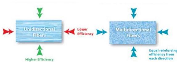
**Fig. 2. FRC reinforcement efficiency according to fiber orientation [24]**
