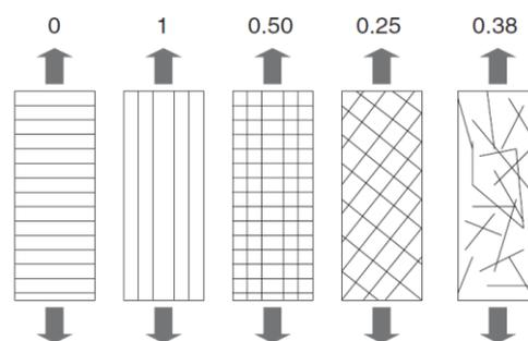
**Fig. 4. FRC reinforcement efficiency according to fiber orientation [42]**
