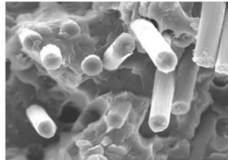
**Fig. 3. SEM Image - Amount of fibers in the polymer matrix [38]**
