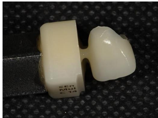
**Figure 4.** The milled crown from polychromatic leucite reinforced ceramic block Empress CAD Multi
