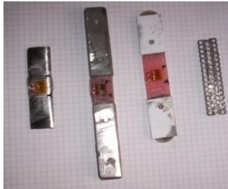
Fig. 7. The specimens instrumented with rosettes TER 125TM
