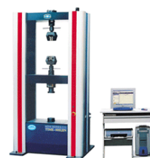
Fig. 4. The universal tensile tests machine WDW-50
