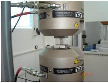
Fig. 5. Cr-Co alloy specimen with holes mounted in the Instron Machine
