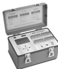
Fig. 3. The Wheatstone bridge, P3 model, manufactured by Vishay
